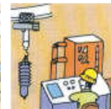
Transportation of fragile items like glass products (No shocks are transmitted to the hoisted load.)
