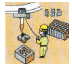
Accurate positioning (The hoisted load does not shake.)
